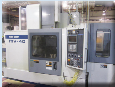
(3) MORI SEIKI MV-40B/APC, SHUTTLE PALLET CHANGER, 31"X16"X20" TRAVELS, 8K RPM, 30 ARM ATC, CT-40, FANUC. 16M, 1994 & 2 -1995'S.
