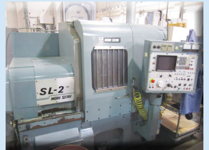
MORI SEIKI SL-2H, 10" CHUCK, 12 STATION TURRET, NO TAILSTOCK, 3" HOLE THRU SPINDLE, FANUC 6T, 1984.
