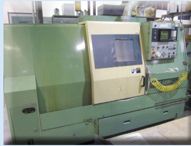
MORI SEIKI SL-25B/500, 10" CHUCK, 2.5" BAR, 10 STATION TURRET, CHIP CONVEYOR, BOX WAYS, FANUC 16T. 1990.
