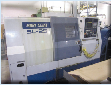
MORI SEIKI SL-25B/500, 10" CHUCK, 2.5" BAR, 10 STATION TURRET, CHIP CONVEYOR, BOX WAYS, FANUC 16T. 1993.
