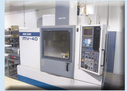
MORI SEIKI MV-40B, 31"X16"X20" TRAVELS, 4TH AXIS ROTARY TABLE - 12" TECNARA W/ TAILSTOCK, 8K RPM, 30 ARM ATC, CT-40, FANUC OMC. 1994.
