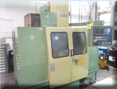
MORI SEIKI MV-40B, 31"X16"X20" TRAVELS, 8K RPM, 20 ARM ATC, CAT-40, RIGID TAPPING, FANUC OMC. 1990.
